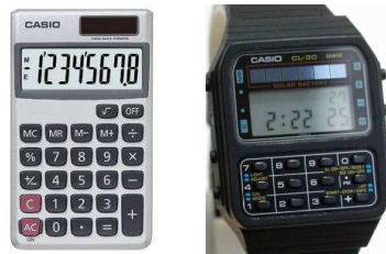
Figure 1.1 Examples of an older generation of electronic devices powered by solar cells such as calculators and digital watches.
