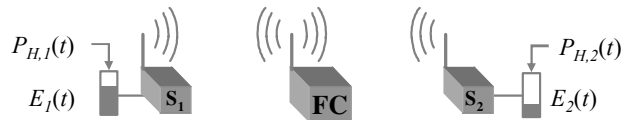
Fig. 1. WSN with a single Fusion Center (FC) gathering data from M sensors, which are provided with energy storage and harvesting capabilities (here, M = 2 ).
